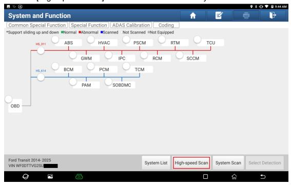
5. Click [ABS (Anti-Lock Brake System)] to access the system.
