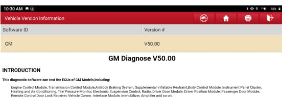
Reading ECU information Reading DTCs Clearing DTCs Reading vehicle running data Vehicle component operation test
