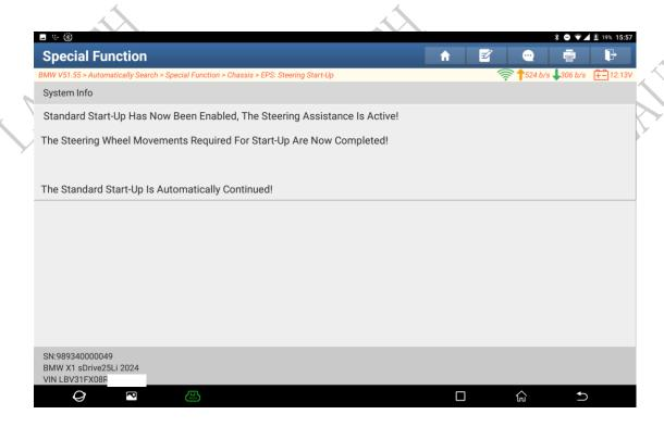
12. Turn the steering wheel according to the previous step prompt. It automatically jumps to the next step when the conditions are met.
