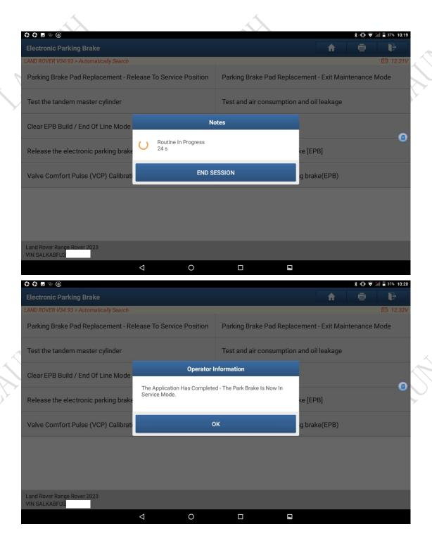
6. Brake pad has been released to service position, it is ready to replace brake pad
