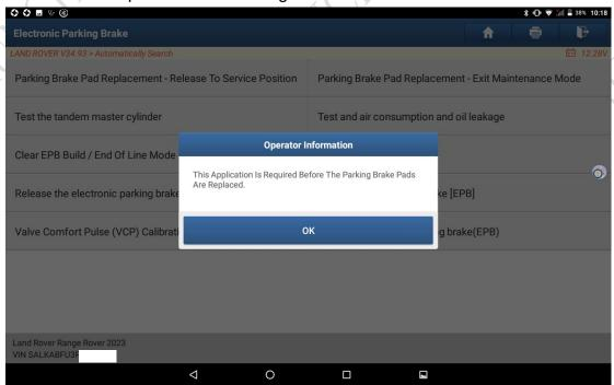
5. Vehicle must keep stationary, no rolling backwards or forwards, battery voltage >12V, if not, it is necessary to charge the vehicle, and then turn on ignition switch according to prompts
