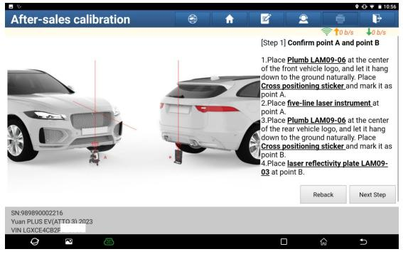
15. Step 2: Connect points A and B with laser, confirm the vehicle center line P, and click [Next Step].
