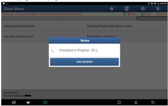
11. Continue to depress and release the brake pedal until no bubble appears in the brake fluid.
