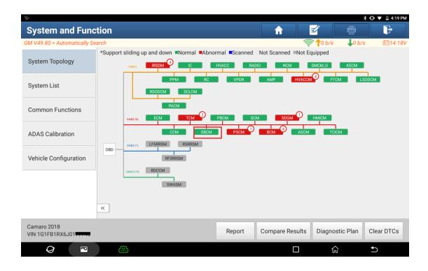
5. Click [EBCM (Electronic Brake Control Module)] to access the system.
