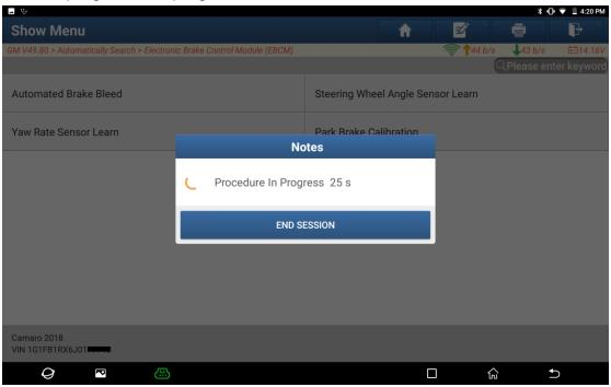
14. Continue to depress and release the brake pedal until no bubble appears in the brake fluid.
