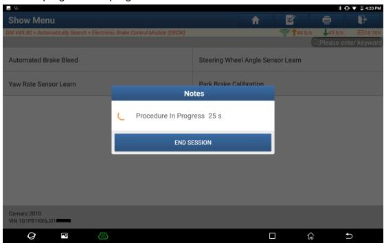
20. Continue to depress and release the brake pedal until no bubble appears in the brake fluid.
