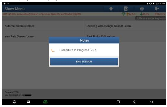
17. Continue to depress and release the brake pedal until no bubble appears in the brake fluid.
