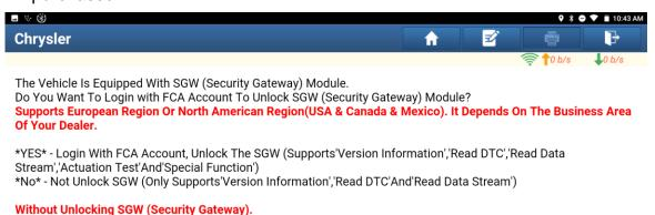
The Diagnostic Software Only Supports'Version Information', 'Read DTC'And'Read Data Stream'Functions.
