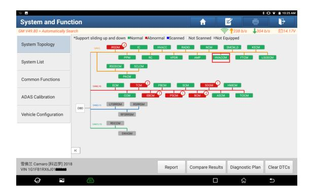
5. Click [HVACCM (Heating Ventilation Air Conditioning Control Module)] to access the system.
