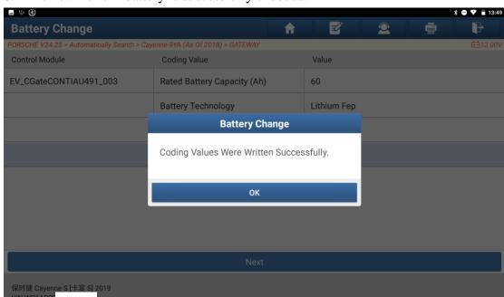
8. The new lithium battery is successfully encoded.
