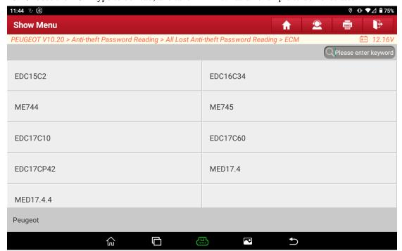
21. After you choose the type, the following prompt box will pop up. If the EEPROM data of MED17.4 has been read and saved, click OK to continue. If the EEPROM data has not been read and saved, go to step 1 to enter the programmer to read and save EEPROM data of the corresponding type.
