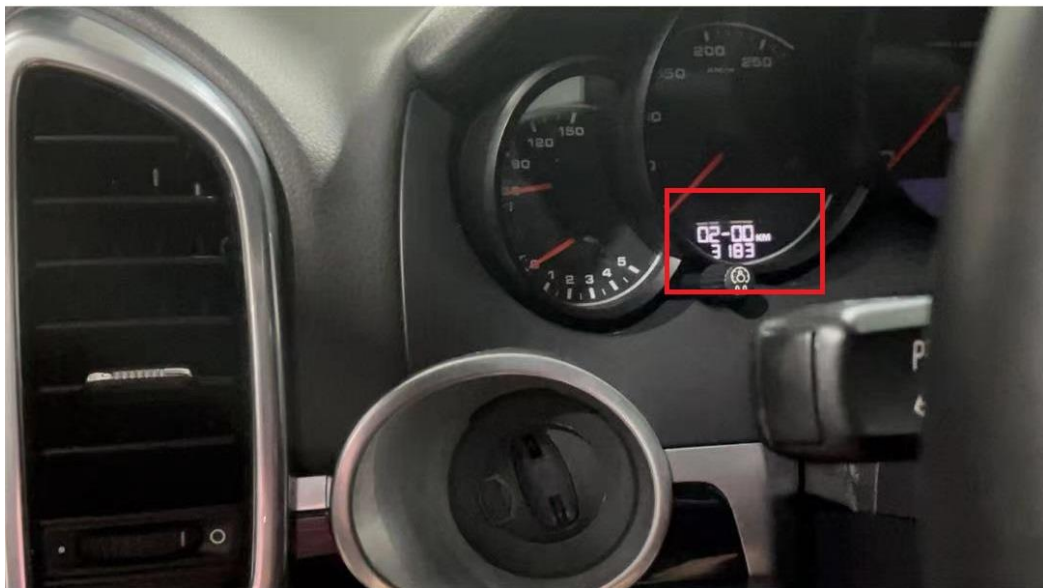
Figure 3-5 Black-screen instrument panel shows 2-0
