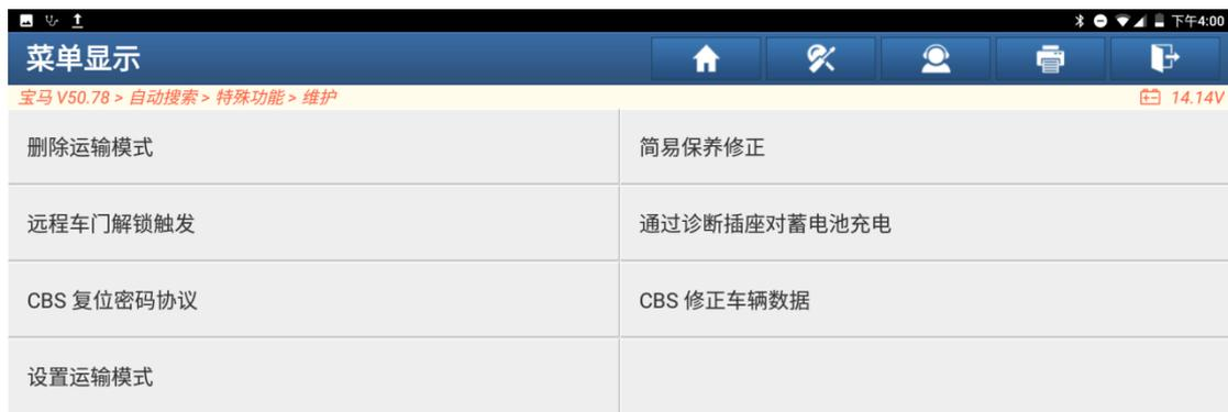
The screenshot shows the '菜单显示' (Menu Display) screen in the Launch diagnostic software. The top navigation bar includes icons for home, search, user profile, print, and share. Below the navigation bar, the breadcrumb path is '宝马 V50.78 > 自动搜索 > 特殊功能 > 维护' (BMW V50.78 > Auto Search > Special Functions > Maintenance), and the battery voltage is 14.14V. The main content area is a table with the following items:
