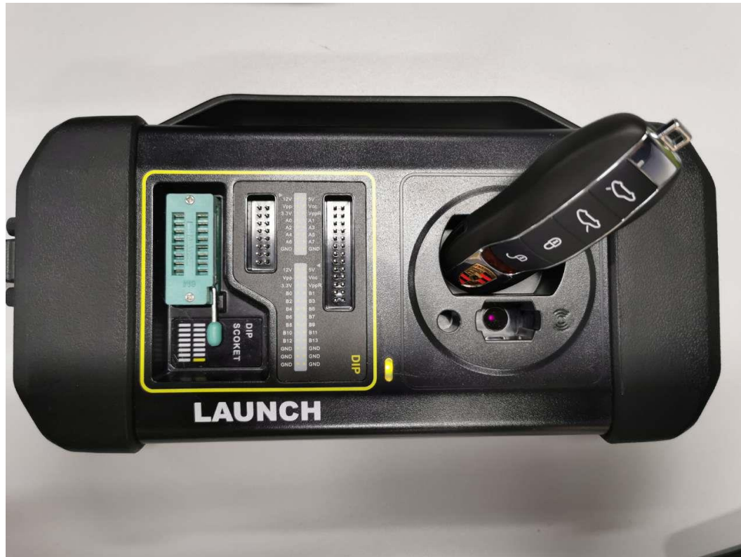
Figure 2-4: The key is placed in the Immobilizer programmer G3
