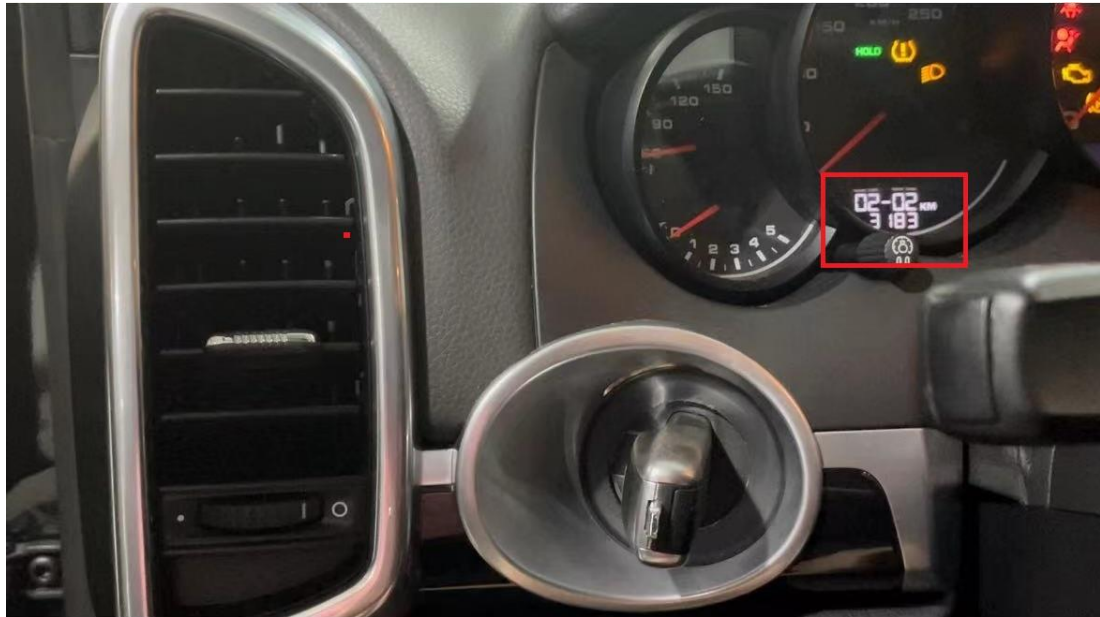
Figure 3-7: The illuminated instrument displays 2-2
