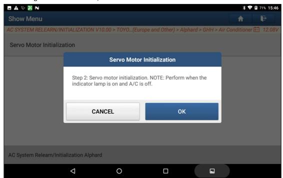
14. The initialization starts, the DEF indicator lamp if off and the automatic indicator lamp in on, if the lamp goes out, the initialization will end.
