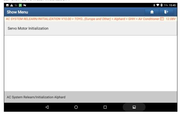
12. Noted that perform the servo motor initialization after replacing the actuator and battery. Click "OK" to continue.
