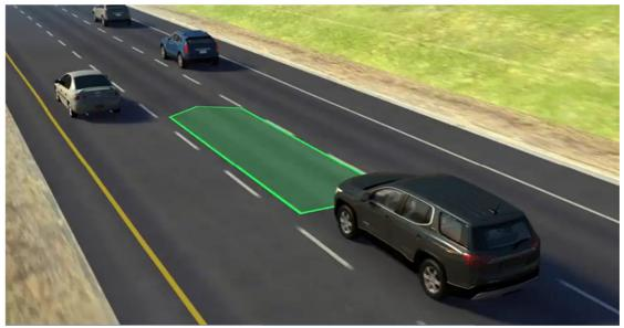
Depending on your vehicle's equipment, Adaptive Cruise Control uses a forward-looking camera, radar or both, to see if there's traffic ahead of you. It senses and responds to a vehicle in front of you in your lane. Your vehicle will speed up or slow down to keep the following distance gap you select – Far, Medium or Near. It can even bring your vehicle to a complete stop.
