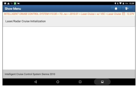
10. This function is used to calibrate the cruise control system, click "OK" to continue.
