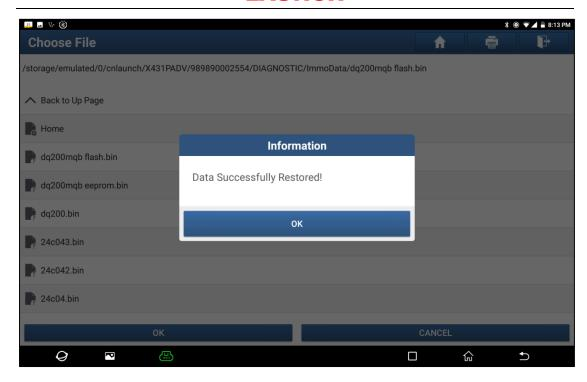
Situation 2: The data of the customer's original vehicle gearbox ECU is unreadable or the data is damaged. In this situation, we need to back up the EEPROM of the ECU for replacement (we call it new gearbox ECU here), and then manually input the original CS code or get the original CS code from the original key.
