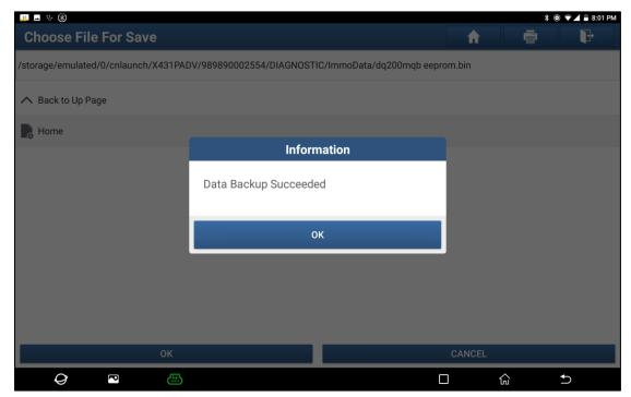
6. Exit the [Special Function], enter the local diagnosis, enter the Volkswagen software, select [Special Function]>>[Anti-Theft Function], click [OK], enter the main menu of the anti-theft system, select [MQB Instrument], click [OK]. Select [Replacement Of Parts]>>[Transmission], click [OK], click [YES] to enter the gearbox replacement page, as shown in the figure:
