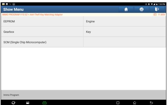
2. Select [Gearbox], and then select Gearbox type according to the specific model, here we choose [DQ200-MQB] to enter the function menu. As shown in the below figure:
