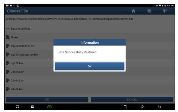
10. Click [Restore FLASH Data] to write the FLASH data of the original vehicle gearbox backed up in step 6 into the gearbox ECU for replacement. The operation steps are the same as step 9, as shown in the following figure:
