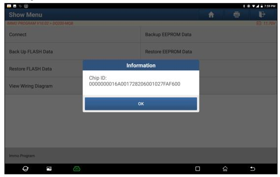
5. Click [Backup EEPROM Data] in this menu interface, read the EEPROM data of the original car gearbox, enter the file name to be saved, click [OK], select the path where the file is to be stored, and click [OK] to save. As shown below:
