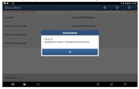
5. Click [Backup EEPROM Data] in this menu, read the EEPROM data of the new gearbox, enter the file name to be saved, click [OK], select the path where the file is to be stored, and click [OK] to save, as shown in the figure below Show:
