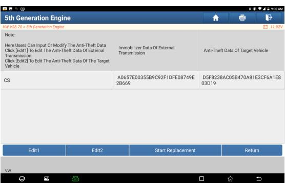
9. Click the [Start Replacement] button, and input the original car's VIN code, power level and CS code of the original car instrument according to the information prompts to complete the gearbox replacement, as shown in the figure:
