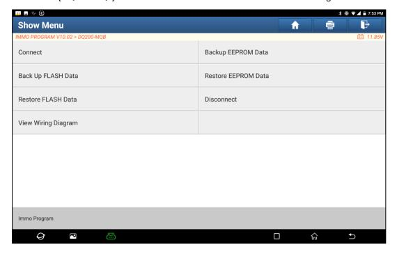
3. Click [View Writing Diagram], then connect the new gearbox ECU with X-431 PRO G3, X-431 Pad V as the below image.
