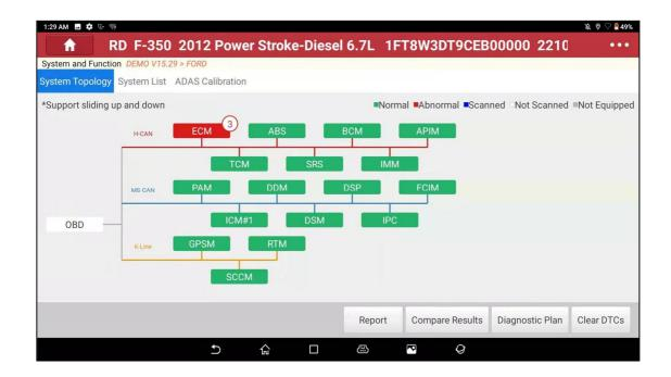
The topology map refers to the physical layout diagram of the interconnection of the vehicle control modules. The topology map does not show the physical connections of the sensors and actuators within each, or the distance between the nodes of each control module, but only shows the relationship between the vehicle control modules in the form of a graph.
