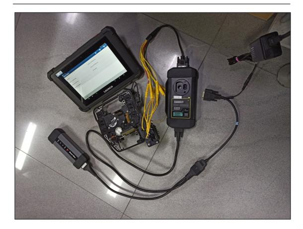
4. Click [Connect], click [OK] after reading the chip ID of the original car gearbox, as shown in the figure:
