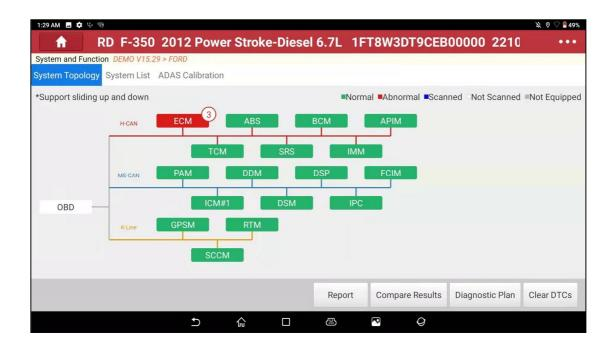
The topology map refers to the physical layout diagram of the interconnection of the vehicle control modules. The topology map does not show the physical connections of the sensors and actuators within each, or the distance between the nodes of each control module, but only shows the relationship between the vehicle control modules in the form of a graph.
