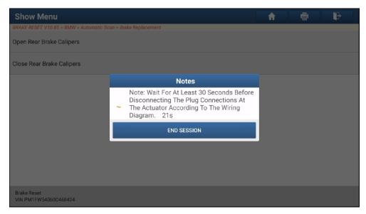
6. After it finished, it pops up reminder to ask you repairs to the EMF can now be carried out according to instruction. We need to change the brake pad now.
