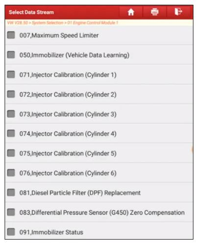
9. Select the injector which you need to programming, here we chose 074 injector Calibration (Cylinder 4).
