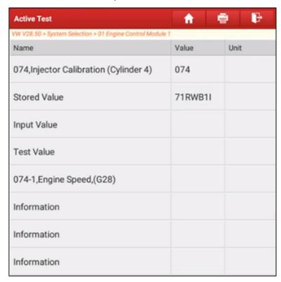
Select input Value, and input the correct number of the injector and click OK.
