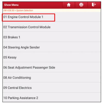
4. Enter "01 Engine Control Module 1" system , the scanner will read ECU memory, and you need to record or print the information on this page which is useful for you to query after-market service center.
