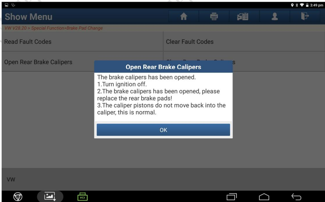
5. After changing the brake pad, select [Close rear brake calipers]. In about 15s, the brake calipers are closed. The warning lamps on the parking brake pressure switch and on the instrument panel may flash all the time. The flash shall stop after cycling the parking brake on and off again.
