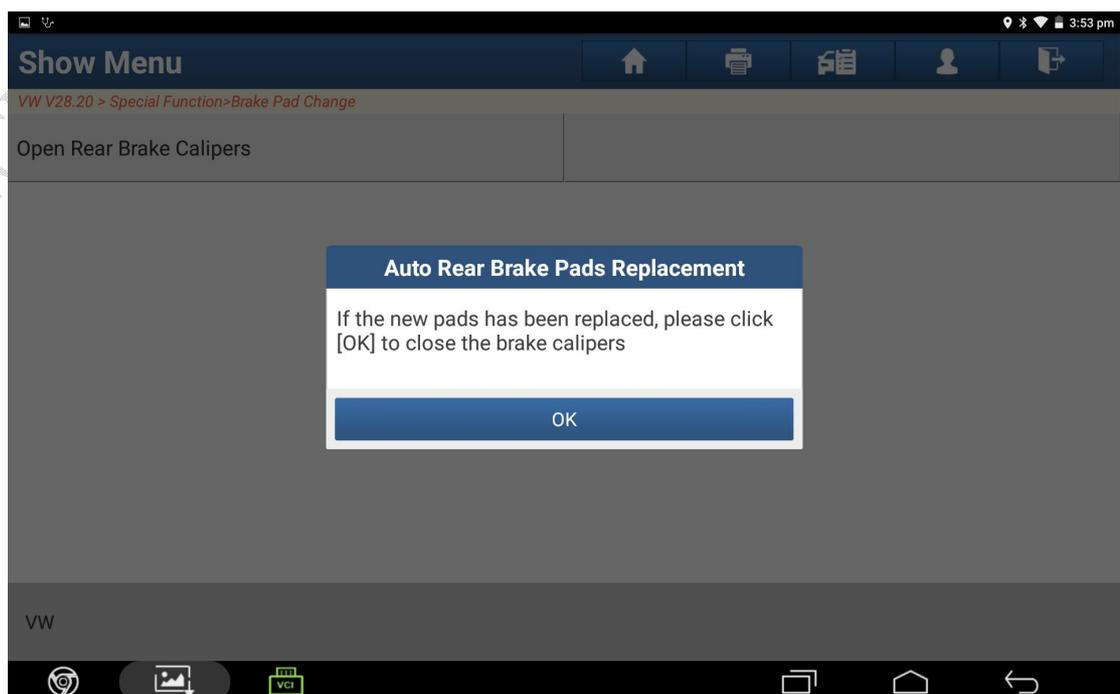
8. After changing the brake pad, select [Close rear brake calipers]. In about 30s, the brake calipers are closed. The warning lamps on the parking brake pressure switch and on the instrument panel may flash all the time. The flash shall stop after cycling the parking brake on and off again.
