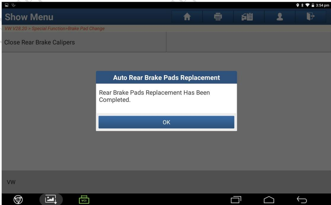
9. After the replacement, select [Clear fault codes] to clear related fault code. If no fault code displayed, it indicates the brake pad has been successfully changed.
