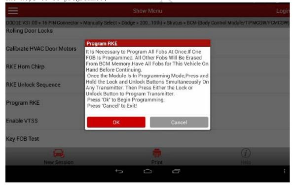
14). Operate according to the hints, and press the Lock button and the Unlock button simultaneously and hold to program
