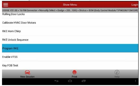
13). Observe the description of the Program Remote Control Key function, and prepare the keys to be programmed;
