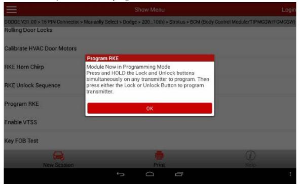
15). After confirmed, it indicates Completed. Press the remote Lock and Unlock buttons. If the door lock motor responds normally, the matching is successful.
