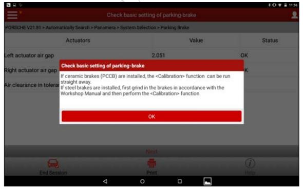
12). After adjusting the gap, select "Break-in" to run in the steel brake pad.
