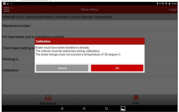
15). After satisfying all the calibration conditions, click OK to perform the "Calibration" of the parking brake. When it prompts the calibration completed, the software operation of replacing the brake pad is completed.
