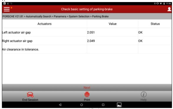
11). Click "Next" to complete the function of "Check the basic setting of parking brake".
