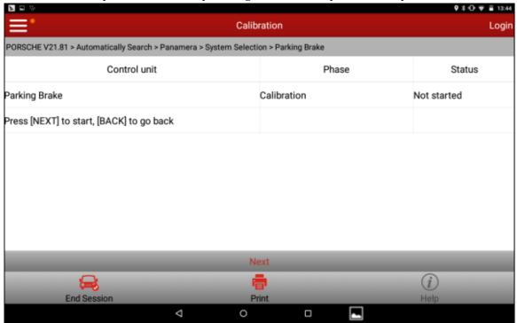
16). Click "Next" to complete and exit. Turn ignition off and on again to test the vehicle. When everything is OK, the procedure of replacing brake pad is completed.
