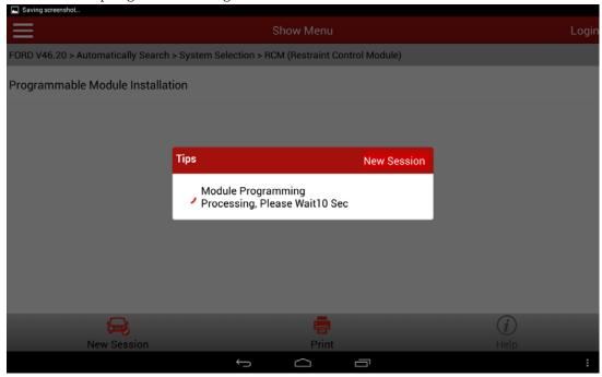
13). After program running is complete, turn the ignition key to OFF (position I) and click OK.
