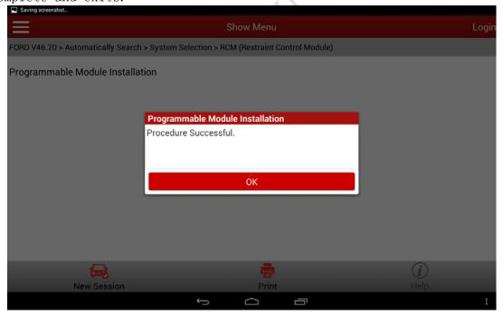
18). After program running is complete, stop and restart the engine to check whether the instrument cluster MIL is on and whether the replaced or initialized module can operate properly.
