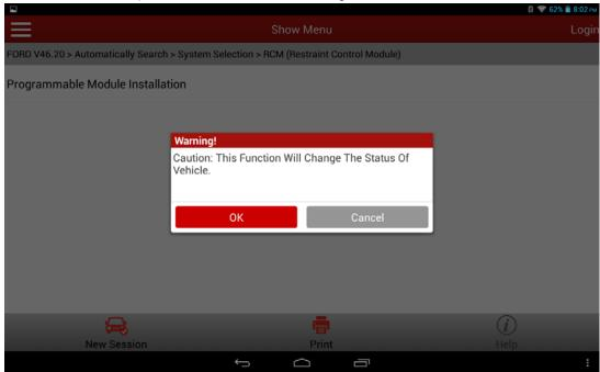
7). Before installing the module, clear the DTCs first and configure an auxiliary power supply to keep the decoder power supply connected.
