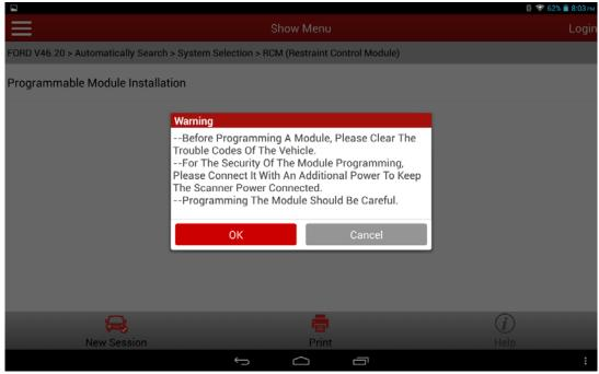
8). Turn the ignition key to ON (position II) and then click OK. The program starts reading old module information.
