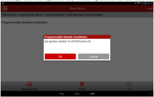
10). After the program completes reading old module information, install a new module. See Figure 5. Ensure that all cables and connectors are correctly connected and the decoder power supply is kept connected. After installation, click OK. The program starts writing new programmable module information.
