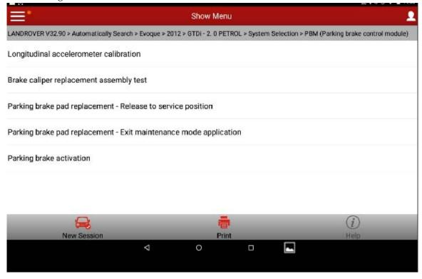
8). Longitudinal acceleration sensor calibration is needed after remove and replace the brake module.
