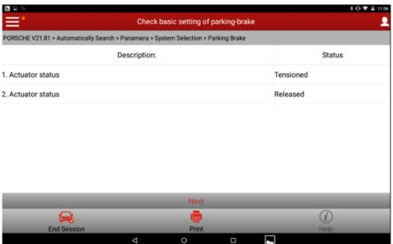
10). Click Next to check the brake pad gap. Note: The standard gap for Porsche panamera (as of 2011) is between 1.9mm-2.4mm. If the gap is out of the range, the status is an exclamation mark. Adjust the gap. If the gap is within the range, the status is a tick.
