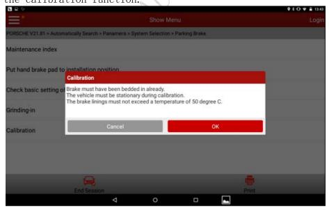
15). After the calibration conditions are met, click OK to perform the calibration function. The calibration is complete.
