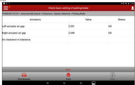
11). Click Next. The function "checking parking brake basic setting" is complete.
