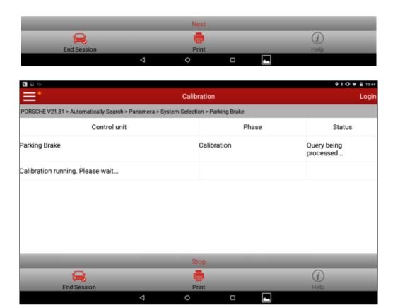
16). Click Next to exit. Restart the engine to drive the car. Everything is normal. The brake pad replacement process is complete.
