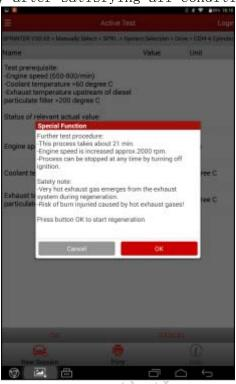
14). Stop the vehicle as prompted and keep the engine run at idle, then click OK to enter the DPF Regeneration.
