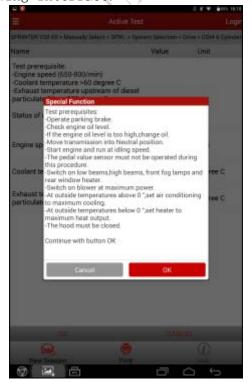
13). Thus, before performing this function or stop at this precondition interface and drive until the exhaust gas temperature is much higher than the required, and keep the engine run at idle to prevent the exhaust gas temperature from decreasing rapidly. Click OK only after satisfying all conditions.
