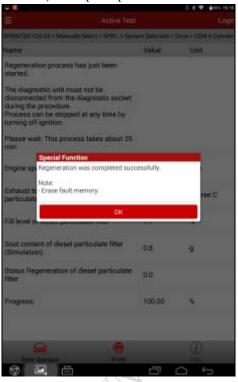
18). If the carbon content displayed in the data stream is still high, check whether there are related sensor DTCs. By now, the particles in the DPF are burned out. The problem of blocking in the DPF is solved. The static DPF regeneration is successfully performed.
