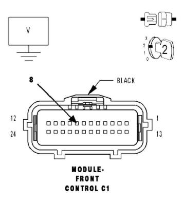
8). (D64) CAN C BUS (-) CIRCUIT SHORTED TO VOLTAGE Measure the voltage between the (D64) CAN C Bus (-) circuit and ground.
