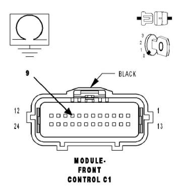
11. (D65) CAN C BUS (+) CIRCUIT SHORTED TO (D64) CAN C BUS (-) CIRCUIT
