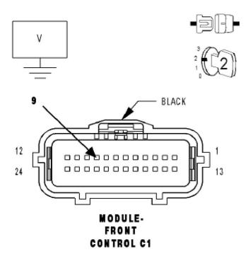
9). (D65) CAN C BUS (+) CIRCUIT SHORTED TO GROUND Turn the ignition off.
