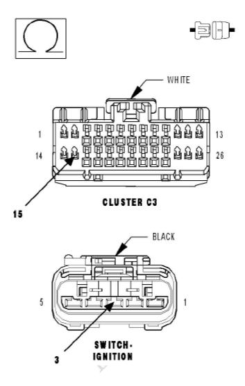
CHECK THE (A106) FUSED B+ CIRCUIT FOR AN OPEN
