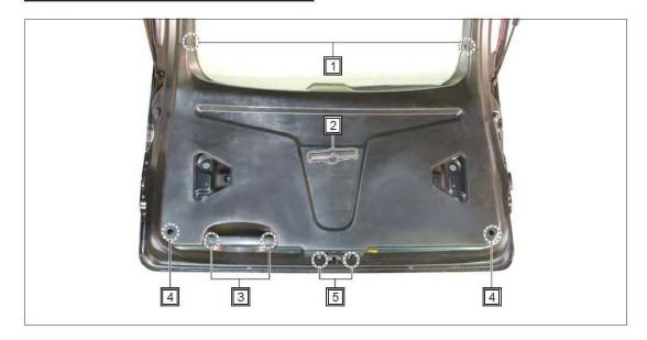
1. Remove the scrivets (LH, RH) and remove the upper trim from the tailgate.
