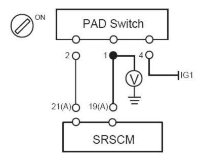
E) Is the measured voltage within specification?
