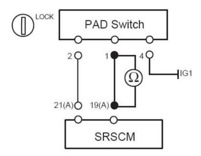
D) Is the measured resistance within specification?
