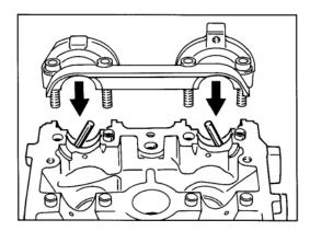
The seal cover may only be used with Special Tool 9234 after the bearing saddle has been tightened.
