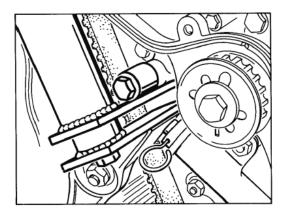
Illustration shows tensioned belt tensioner locked with Special Tool 9530, assembly tool (pin).
