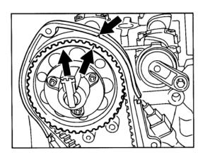
TDC mark on flywheel (center notch) with engine fitted (double-mass flywheel).
