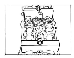
6. Fit camshaft bearing saddles and bearing covers. The bearing saddles or covers are machined as a unit with the cylinder head and must always be fitted as a unit. Observe correct identification character and matching number. Tighten bearing saddles or covers to 20 Nm (15 ftlb).
