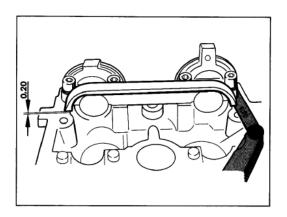
Oil sealing cover lightly and press in manually. Tighten bearing saddle to specified torque.
