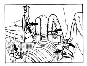
Remove oil dipstick. Pull vacuum non-return valve from brake booster. Remove coolant hose between radiator and cylinder head from breather flange. Undo intake rail at lefthand engine mount. 10. Remove bracket for oxygen sensor connector from intake rail. Loosen breather hose at oil separator and coolant hoses at connecting flange and pull off. Remove wiring harness bracket from connector flange.
