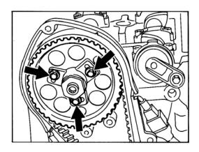
4. Undo central camshaft bolt, using a suitable retainer to keep the camshaft from turning. Rotate engine against the sense of rotation until the camshaft gear is against the stop within the woodruff key groove.
