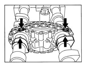
Oil bearing surfaces of camshaft, cylinder head and cams. Fit camshafts with assembly saddles, Special Tool 9248, used in conjunction with tensioning pins of Special Tool 9226, to cylinder head.
