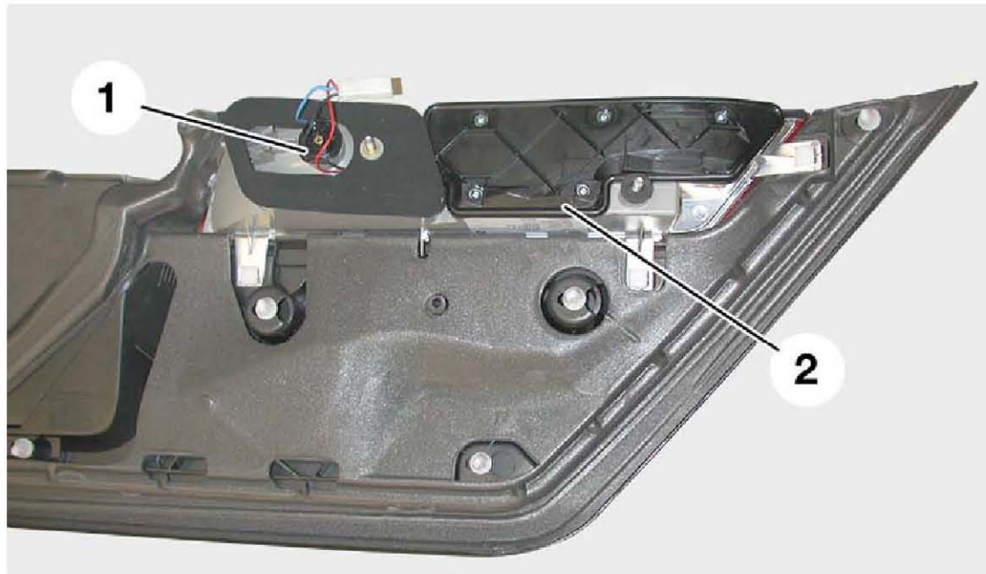
Fig. 48: Rear view, lights in the rear lid trim panel
