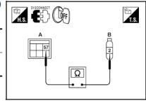
Check continuity between the IPDM E/R harness connector (A) and license plate lamp connector (B).
