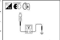
7. With the parking lamps ON, check voltage between the license plate lamp connector and ground
