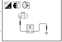
With the parking lamps ON, check voltage between the rear combination lamp connectors and ground.
