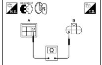
4. Check continuity between the IPDM E/R harness connector (A) and the rear combination lamp harness connector (B).
