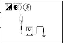
Check continuity between the license plate lamp harness connectors and ground.
