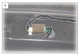
4. Disconnect the ground (a) and heated wiring cable (b) from the tailgate. Then, remove the wiring assembly.
