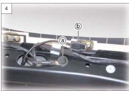
Release the fixing clips and remove both shock absorbers.
