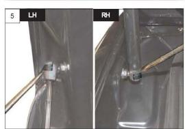
Unscrew two hinge bolts (LH/RH, 10 mm) and remove the tailgate assembly.
