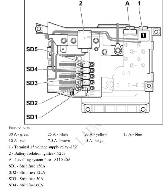
Relay and fuse carrier under driver seat
