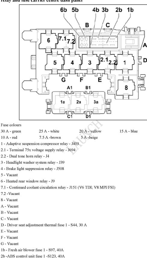
relay and fuse carrier centre dash panel
