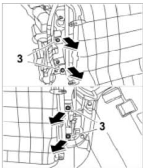
旋开热交换器托盘的紧固螺钉
