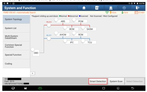
5. Click [AHCM (Auxiliary Heater Control Module)] to access the system.
