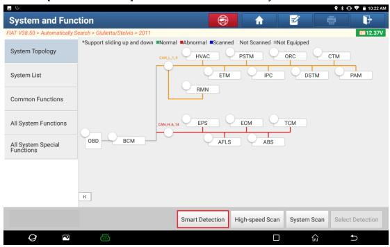
8. Click [ABS (Anti-Lock Braking System)] to access the system.
