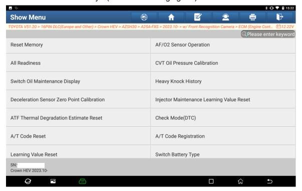
4. Use this function after replacing the automatic transaxle assembly and valve body assembly. Click OK. (See the following figure.)
