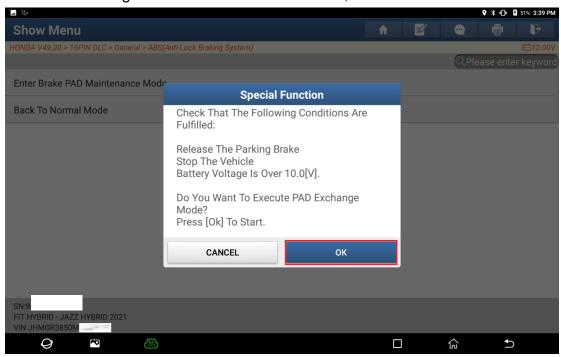
10. Please wait while the vehicle switches to the brake pad maintenance mode.
