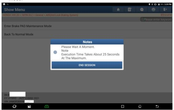
11. After switching to the maintenance mode, perform brake pad maintenance or replace the brake pad. After completion, click OK.
