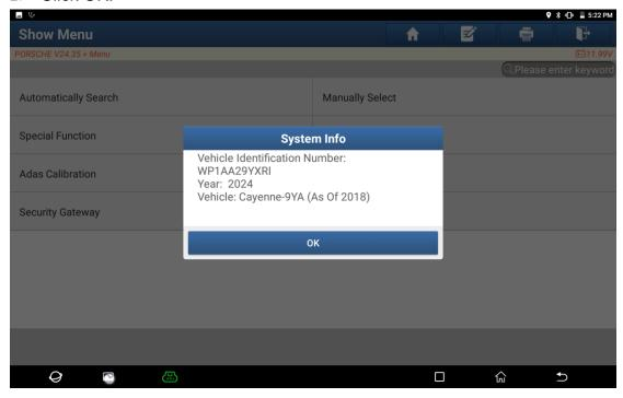
3. Click OK. This car model (2024MY) is equipped with an online second-generation security gateway (SFD), which needs to be unlocked before the service function can be performed.
