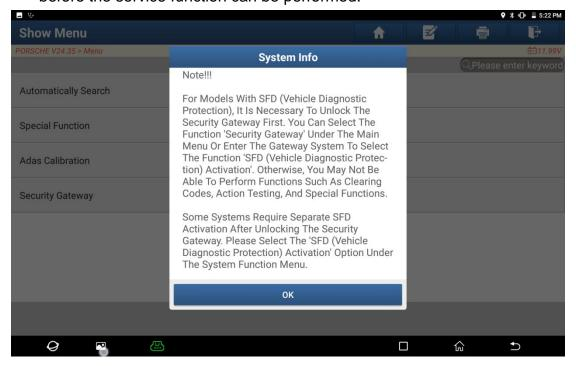
4. [For the second-generation gateway SFD, you need to unlock the security gateway system first, and then unlock the instrument cluster]. First choose [Security Gateway].
