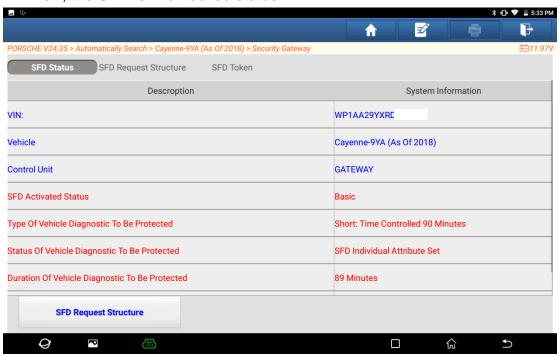
18. After the security gateway is unlocked, continue to unlock the SFD in the instrument cluster. Exit the current interface and click [YES].
