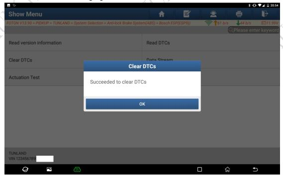
After DTC clearing, the ESP lamp on the instrument panel goes out, indicating that the calibration is successful.
