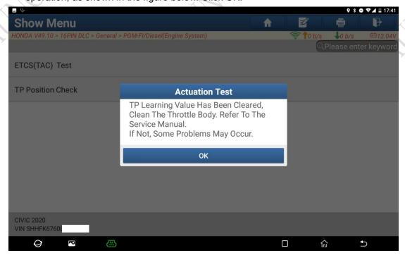
5. Start the engine. If the engine speed is unstable, follow the steps in the figure below to learn the idle speed.
