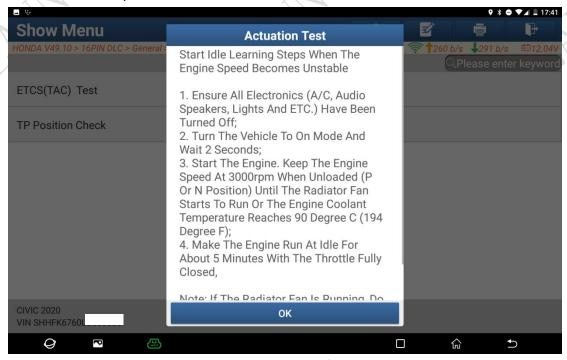
6. The program will guide the execution of the "ECM/PCM reset function", as shown in the figure below. At this time, start the engine first and check whether the engine idle speed is normal. If it is normal, choose CANCEL and the idle speed learning process is completed. If it is not normal, choose OK when the execution conditions in the figure are met.
