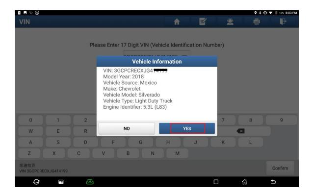
3. Click the Smart Detection button with PAD V to scan all systems of the whole vehicle, then click [ECM (Engine Control Module)] to enter the system;
