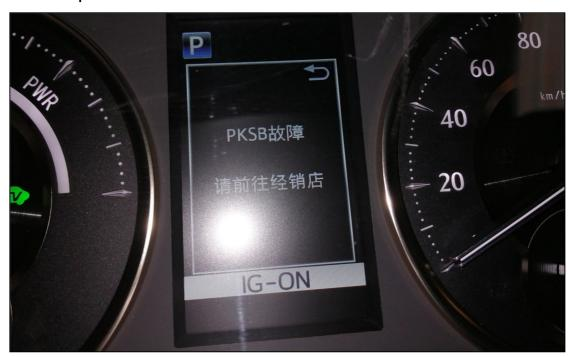
After replaced front and rear bumpers, odometer shows PKSB fault.
