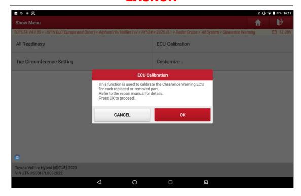
5. Select the parts which have been replaced or removed to proceed. Click [OK] to select.
