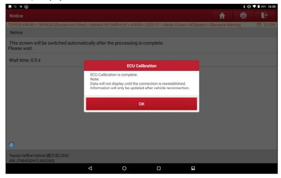
25. Back to clearance warning system and read DTC, no trouble code.
