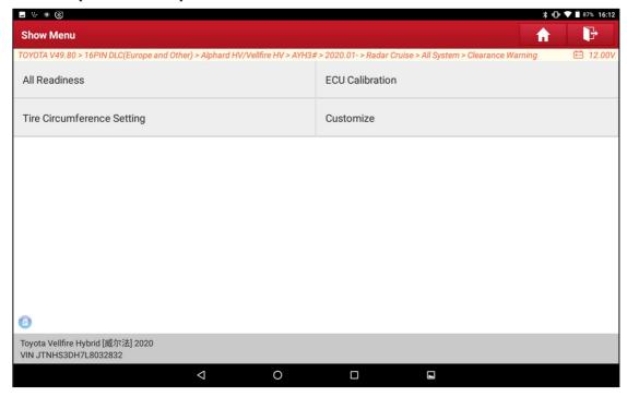
4. ECU Calibration is used to make a setting of necessary clearance warning ECU calibration for each replaced or removed parts, read the ECU calibration introduction carefully, and click [OK] to continue.
