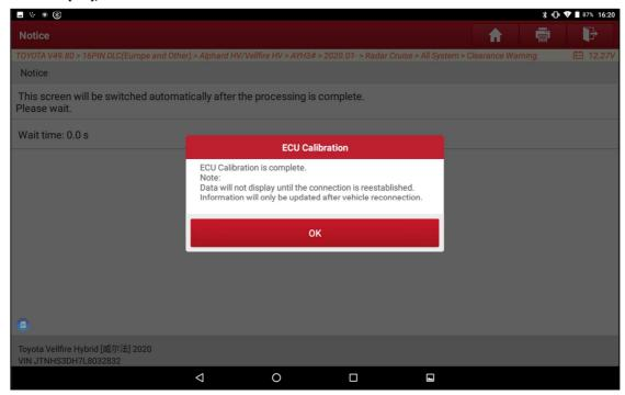
13. Now we are going to calibration rear sensor and bumper, select [ECU Calibration].
