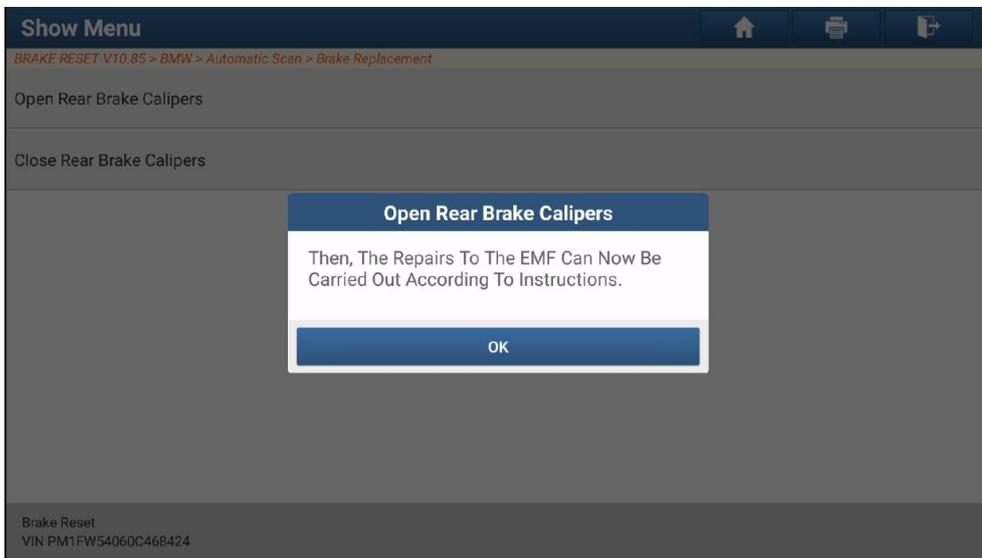
7. After finished change brake pad, click ok to continue, and switch on ignition.
