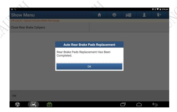
9. After the replacement, select [Clear fault codes] to clear related fault code. If no fault code displayed, it indicates the brake pad has been successfully changed.
