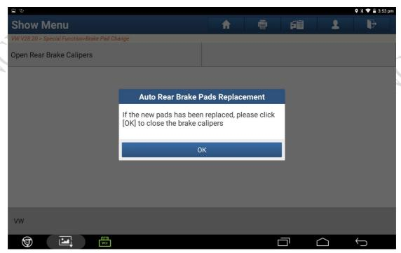
8. After changing the brake pad, select [Close rear brake calipers]. In about 30s, the brake calipers are closed. The warning lamps on the parking brake pressure switch and on the instrument panel may flash all the time. The flash shall stop after cycling the parking brake on and off again.
