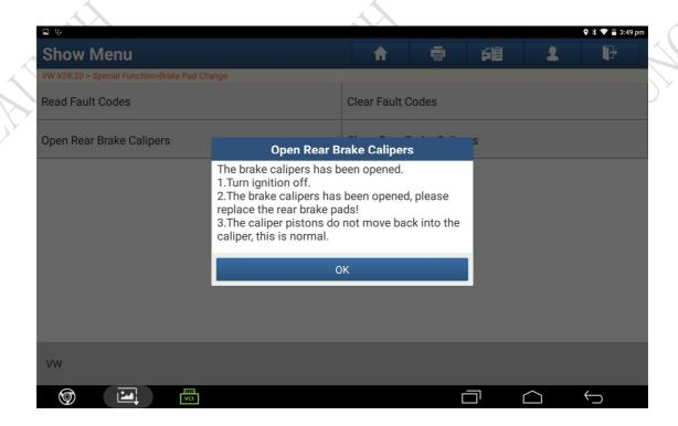
5. After changing the brake pad, select [Close rear brake calipers]. In about 15s, the brake calipers are closed. The warning lamps on the parking brake pressure switch and on the instrument panel may flash all the time. The flash shall stop after cycling the parking brake on and off again.
