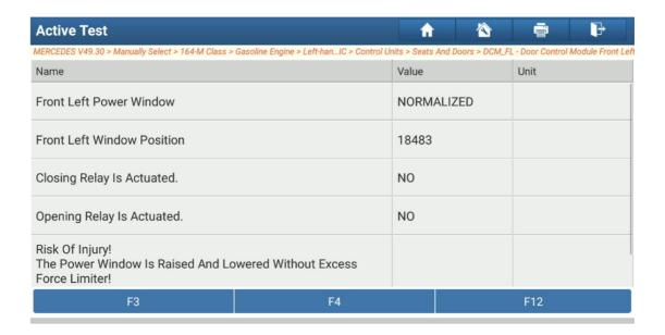
15. After step14, exit action test and clear DTC, then exit software, turn off ignition. FL power window become normal.
